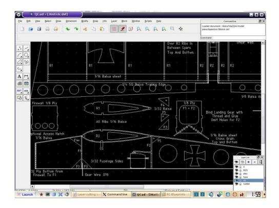
The ribs here are to be setup to be cut on a sheet of balsa 3"x36". The first thing I do is copy the rib to a blank page into Qcad. I then create a second temporary layer to draw the 3"x36" balsa sheet on, to use as a reference. This is done so you can visually see that the parts actually fit on the sheet. Create this virtual Balsa sheet in the 00 or home position.
