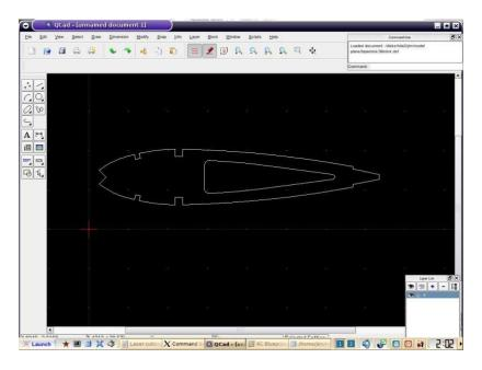
Now that we can see where the ribs go, we need to copy and paste multiple copies into position on our "balsa". For this model we need 8 of the R1 ribs. Again take note of the grain and try to save material where you can. Leave 1/8" minimum around the sheet perimeter and between the parts.
