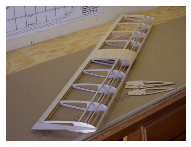
Lets touch on labeling parts. What I do is setup the text in another layer on the Cad drawing. This will be on another layer separate from the ribs. With the software I'm using it's easier to label the part first, adjust the power on the laser, then cut the parts out. There are services that can label and cut in one pass. Again check with your laser cutting service to see what they require..
