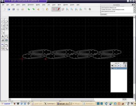
Once the ribs are in position, the "balsa" on our temporary layer can be removed. Save your file and it's basically ready to be sent to the cutter. Remember one sheet one file. If you have two different sheets to cut make two files.
